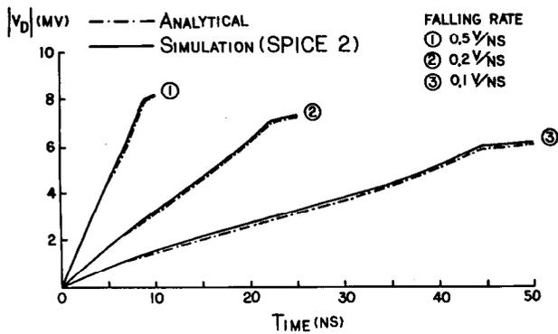
Fig. 3. Comparison of the analytic and computer simulated transient responses for three different gate voltage falling rates. The parameters for Figs. 3 and 4 are  $V_S = 0$ ,  $C_L = 2$  pF,  $V_{T0} = 0.60$  v,  $W = 4$   $\mu$ m,  $L = 3.3$   $\mu$ m,  $L_D = 0.35$   $\mu$ m, and  $\beta = 30.3$   $\mu$ A  $\cdot$  V<sup>-2</sup>.
