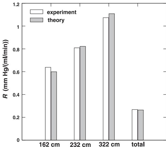
Fig. 6. Resistance ( $R$ ) to the flow of each vessel of the parallel association and total equivalent resistance. The experimental values were derived from measurements shown in Fig. 5.
