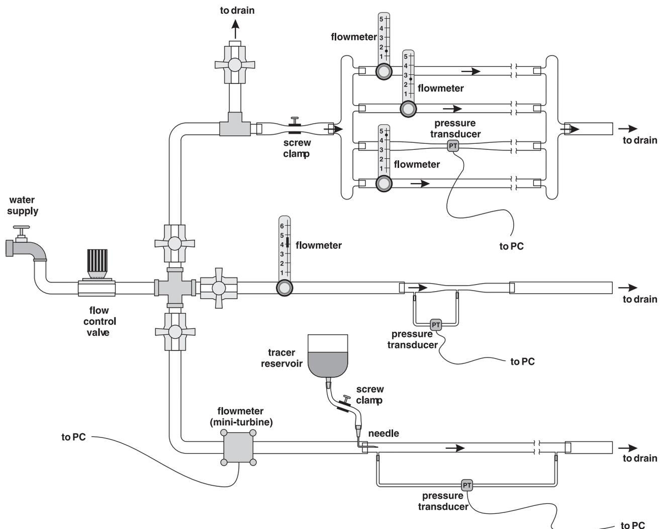
Fig. 1. Schematic picture of the setup used in the experiments. PC, personal computer; PT, pressure transducer.
