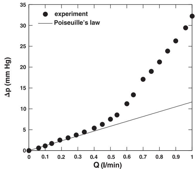
Fig. 2. Experimental pressure drop ( $\Delta p$ ) in a horizontal vessel as a function of the flow rate ( $Q$ ). Poiseuille's law ceases to be verified above 0.5 l/min [Reynolds number ( $Re$ )  $\approx 2,100$ ], approximately, when the flow is no longer laminar but turbulent.
