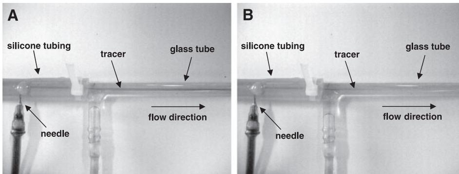
Fig. 3. Laminar and turbulent flow visualization by means of a tracer injection. *A*: laminar flow corresponding to  $Re \approx 1,700$ . The injected tracer keeps its identity without mixing with the surrounding fluid. *B*: turbulent flow corresponding to  $Re \approx 2,500$ . The injected tracer becomes immediately mixed with the surrounding fluid, thus losing its identity.
