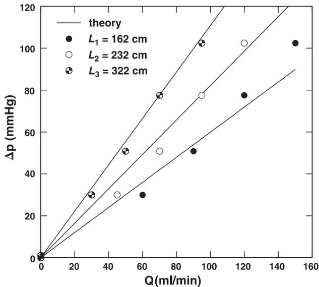
Fig. 5. Experimental pressure drop along the three vessels (of length  $L$ ) associated in parallel as a function of the flow rate. The solid line corresponds to the pressure drop according to the theory, which includes the pressure drop due to viscous losses (Poiseuille's law) and the local pressure drop due to the presence of the flowmeter.
