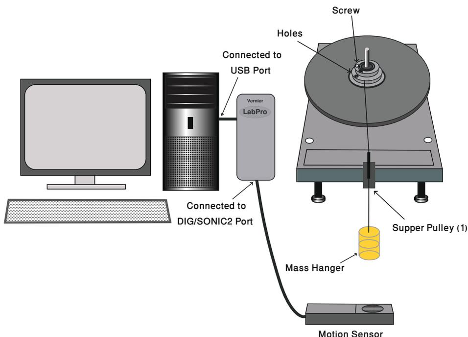
Figure 5: Experimental arrangement for frictional loss measurement.
