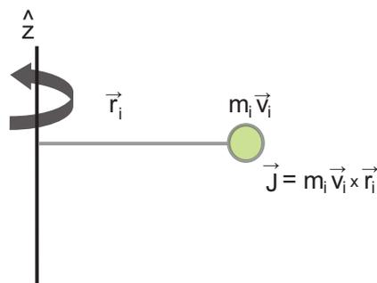
Figure 1: A representative particle rotating about the z-axis;  $m_i v_i$  is the linear momentum and  $J$  is the angular momentum.
