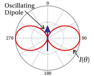
**Figure 3.7** The intensity radiation pattern of an oscillating dipole as a function of angle. Note that the dipole does not radiate along the axis of oscillation, giving rise to Brewster's angle for reflection.
