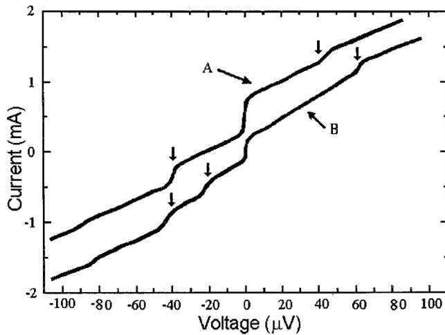
FIG. 3. Shapiro steps on the  $I$ - $V$  curve of the three JJ SQUID under two different external magnetic fields. In curve (A), a giant Shapiro step was observed, denoted by an arrow. In curve (B) two normal steps were observed in the negative sweep and one giant Shapiro step was observed in the positive sweep.
