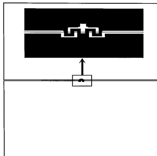
FIG. 1. Picture of the dc SQUID with three JJs in series in each arm. Arrow points to magnification of the SQUID loop (white). A black line indicates the position of the bicrystal boundary. The six junctions form when the strips of YBCO film cross the bicrystal boundary.
