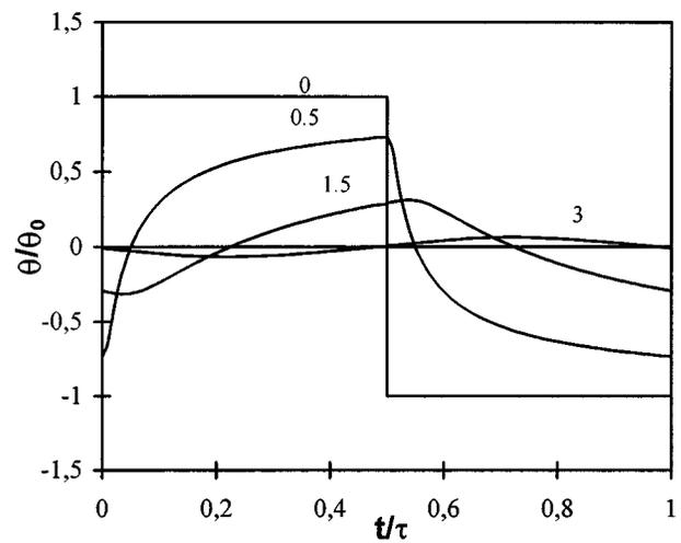
Fig. 1. Theoretical progressive harmonization of the wave at different distances from the sample origin.
