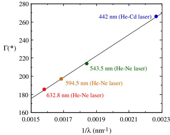
**Figure 7.** Retardation angle  $\Gamma$  as a function of  $1/\lambda_0$  and linear fit.
