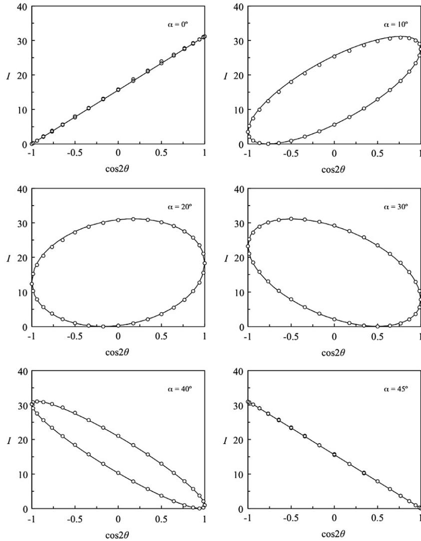
**Figure 4.** Measured intensity as a function of  $\cos 2\theta$  for a wavelength of 632.8 nm: experimental measurements (dots) and theoretical values (continuous line) obtained considering  $I_0 = 15.6 \pm 0.4$  (au) and  $\cos \Gamma = -0.995 \pm 0.005$  in equation (13).
