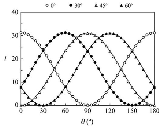
**Figure 6.** Measured intensity as a function of  $\theta$  for different values of  $\alpha$  and a wavelength of 632.8 nm.
