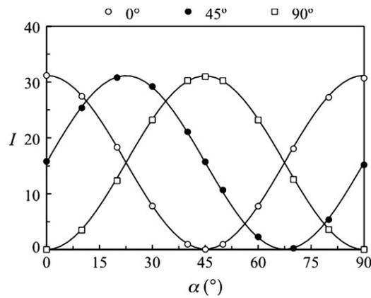
**Figure 5.** Measured intensity as a function of  $\alpha$  for different values of  $\theta$  and a wavelength of 632.8 nm.
