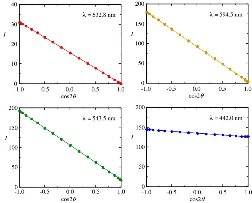
**Figure 3.** Measured values of the intensity (dots) as a function of  $\cos 2\theta$  for  $\alpha = 45^\circ$  and linear fit (continuous lines) for the four wavelengths considered.
