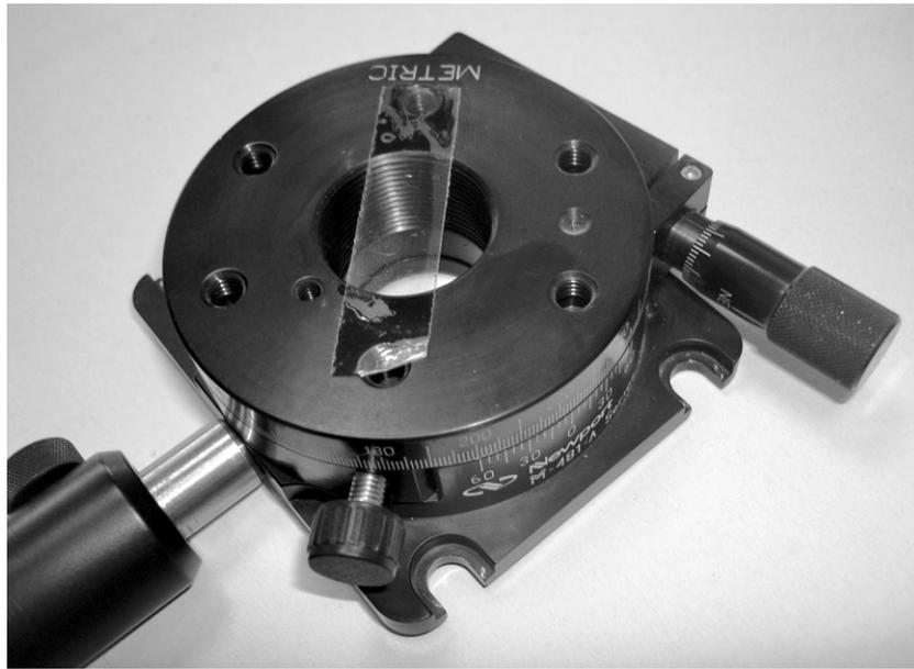
**Figure 2.** Photograph of the cellophane on the rotation stage.
