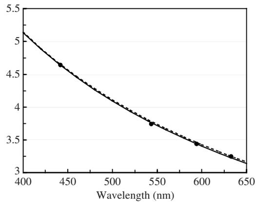
**Figure 8.** Birefringence versus the wavelength of a single cellotape layer. Experimental (dots), fitting considering that  $\Delta n$  is not a function of the wavelength (dashed line) and fitting considering that the wavelength dependence of  $\Delta n$  is the Cauchy-type equation (continuous line).
