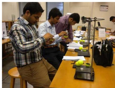
**Teachers, in a workshop, measure the moment of inertia in a torsional pendulum, reminiscent of Cavendish's famous experiment to measure earth's inertia.**
