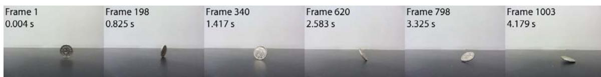
High-Speed Video of a coin revolving and precessing about different axes. Shot at 240 frames per second.
