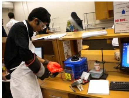
**A student measures the latent heat for vaporizing nitrogen.**
