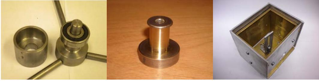
*Bearing fixture assembly (left), Dielectric heater copper base (middle) and the XRF Shielding box (right)*
