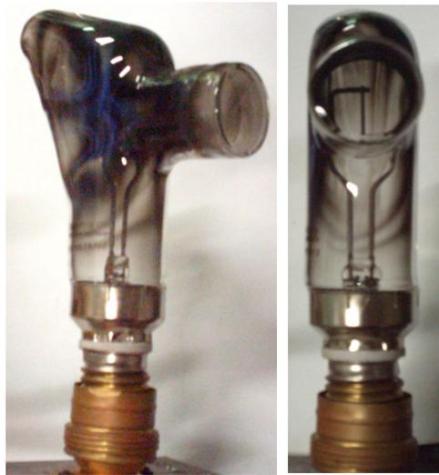
Figure 5. Photograph of the standard tungsten ribbon lamp.
