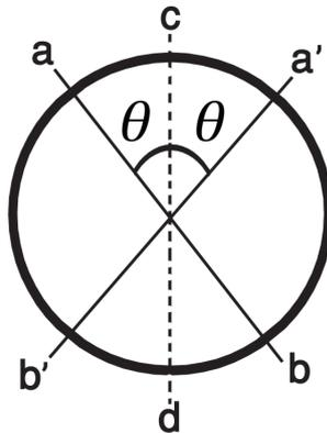
Figure 2: Conceptual working of a half-wave plate.  $ab$  is the plane of polarization of the incident light,  $cd$  is the fast axis of the half-wave plate and  $a'b'$  is the plane of polarization of the transmitted light which has been rotated by the half-wave plate.
