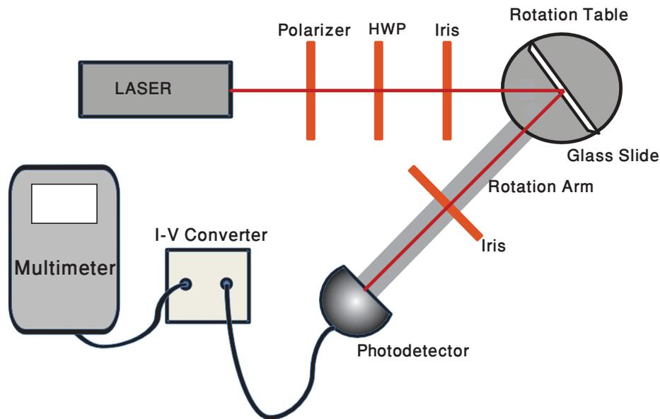
Figure 1: Schematic of the experimental setup. The red line represents the conceived path of the laser beam.
