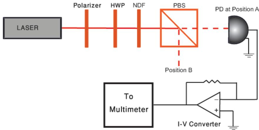
Figure 1: Setup for the polarizing beam splitter (PBS) experiment. The red line shows the perceived light path.
