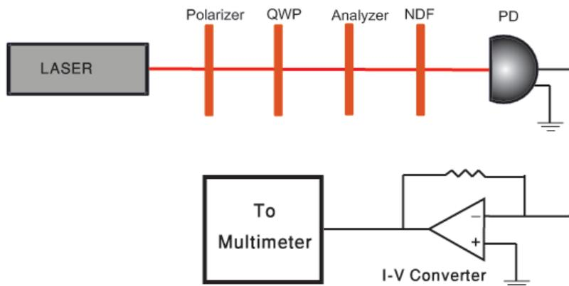
Figure 2: Setup for producing and analyzing circular and elliptical polarizations.
