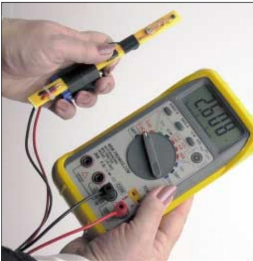
**Fig. 3.** Probe may be held in one hand and used to measure the magnetic field near a magnet. An inexpensive multimeter provides voltage readout.
