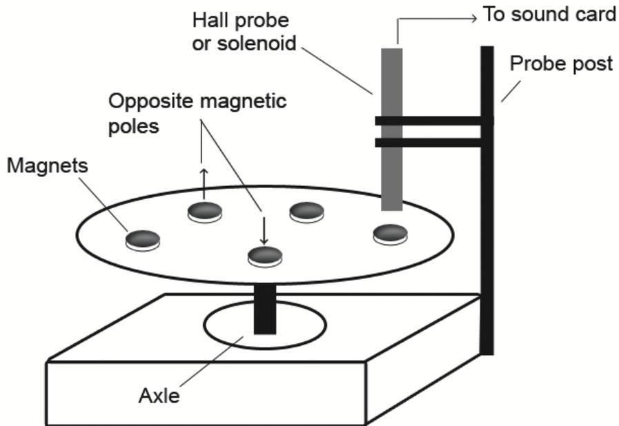
Figure 6: Setup of the experiment. The magnets can be perched in two configurations, with their magnetizations pointing up or down.
