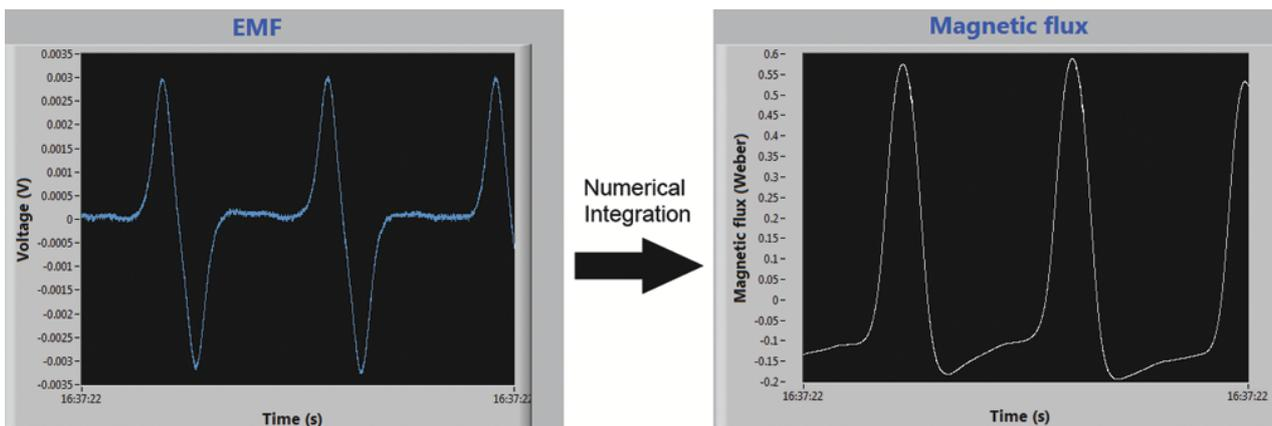
Figure 8: (a) EMF induced in the solenoid as the magnet passes below the solenoid and (b) Shows the numerical integration of the EMF.
