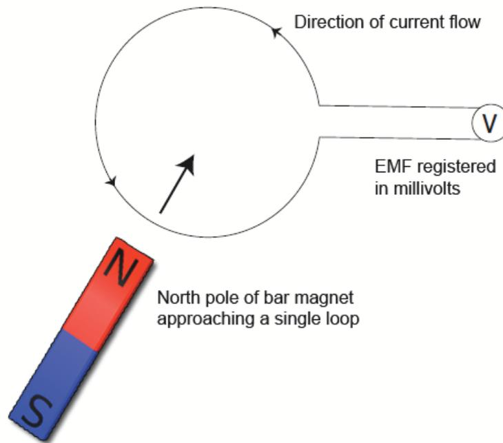
Figure 1: Principle of electromagnetic induction. As a dipole (such as a magnet) is pulled towards a loop of wire, the flux through the loop changes inducing an EMF and current through the loop.
