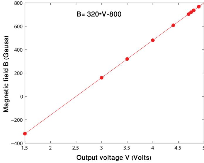
Figure 5: Calibration curve of the Hall sensor employed in the experiment
