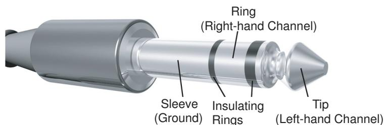
Figure 7: TRS stereo jack connector.
