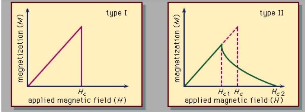
Figure 2: Magnetization vs Magnetic field for type I and II superconductors[3]
