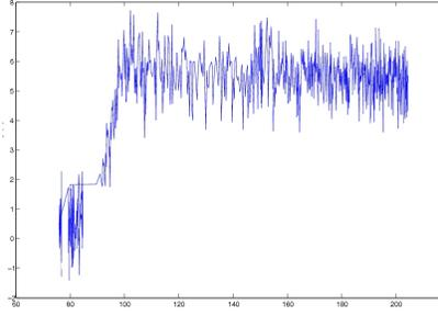
Figure 3: Resistivity Measurement, On y-axis is potential difference in mV and on x-axis temperature in K
