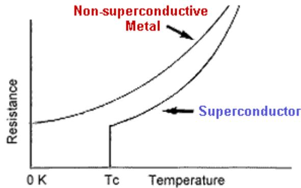
Figure 1: Resistance vs Temperature for a Super-conductor and non-superconductive metal [2]
