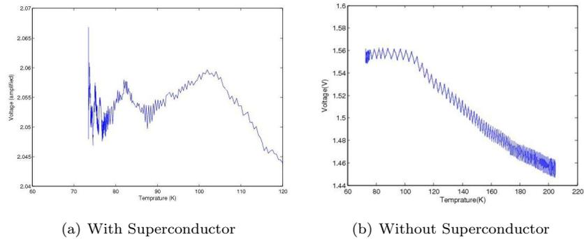
Figure 6: Second Approach: Temperature vs Output Voltage of GMR sensor
