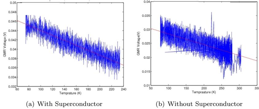
Figure 5: Results of the 1st approach: Temperature vs Output Voltage of GMR sensor
