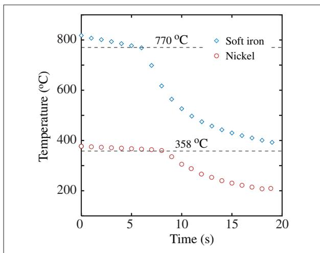
**Fig. 2. Cooling curves for the iron and nickel spheres. The change in the slope occurs when the sphere jumps off the thermocouple and onto the magnet, indicating the corresponding Curie temperature (horizontal lines).**
