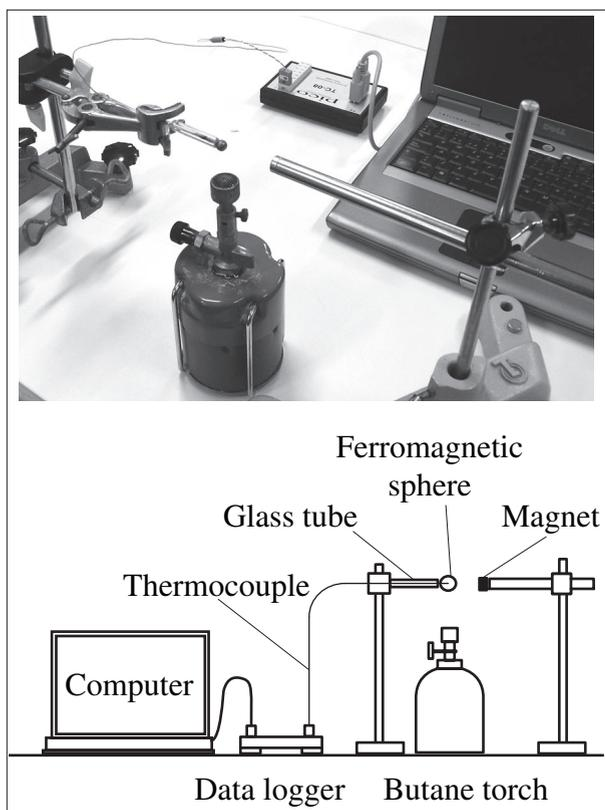
**Fig. 1.** Photo and schematic of the experimental setup used to determine the Curie temperature of iron and nickel. The end of a Type K thermocouple is inserted into a small hole in the sphere, the temperature of which is recorded by means of a data logger connected to a PC.
