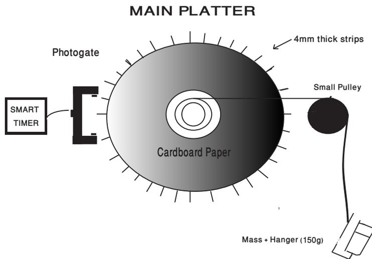
Figure 6: The new setup, with the marked cardboard pasted on the Main Platter.
