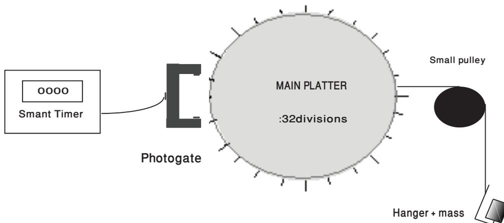
Figure 4: The setup, with the Main Platter calibrated
