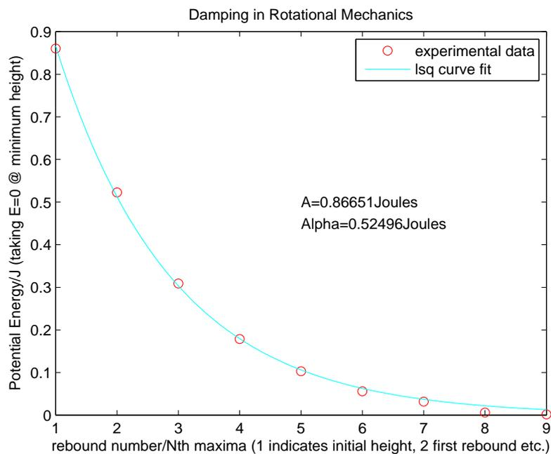
Figure 7: Final graph generated with curve fitting.
