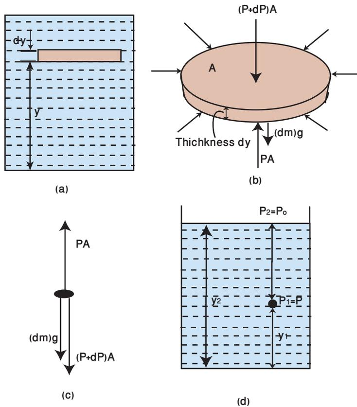
Figure 1: A static fluid. (a) Small element at rest, (b) forces acting on small element, (c) free body diagram, and (d) a fluid with top surface open to the atmosphere.
