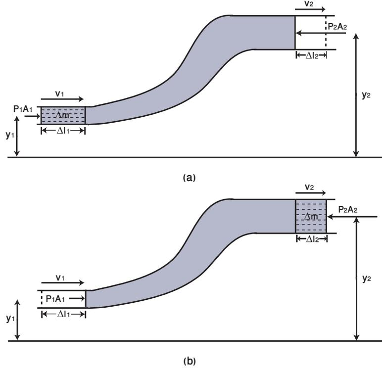
Figure 3: A fluid is flowing through a pipe from position (a) to (b). The net effect is the transfer of the element ( $\Delta m$ ) from left to the right end.
