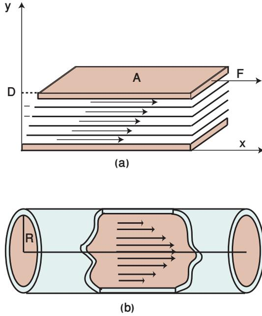
Figure 2: Fluid flow. (a) A fluid filling the space between two plates separated by a distance  $D$ , (b) fluid flowing through a cylindrical pipe with radius  $R$ .
