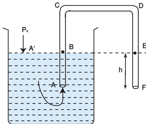
Figure 5: A schematic diagram of a siphon.
