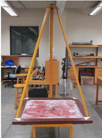
(c) Arrangement showing placement of camera and the tripod over the carrom board.
