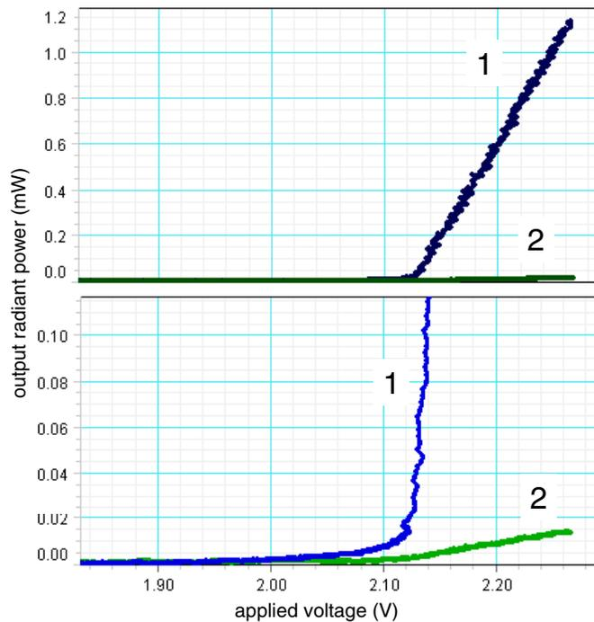
**Figure 5.** Optical output power versus applied voltage after passing a polarizer set for the maximum (1) and minimum (2) signals. The vertical scale of the bottom graph is ten times enlarged. Above the lasing threshold, the maximum-to-minimum ratio is nearly 100.
