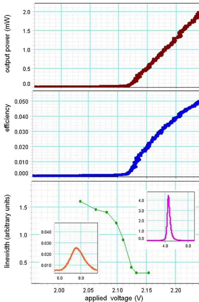
**Figure 4.** Characteristics of the laser diode close to the lasing threshold: the radiant output power, efficiency and emission line width. In the insets, the horizontal scale is nearly the same, while the vertical scales differ by a factor of 100.
