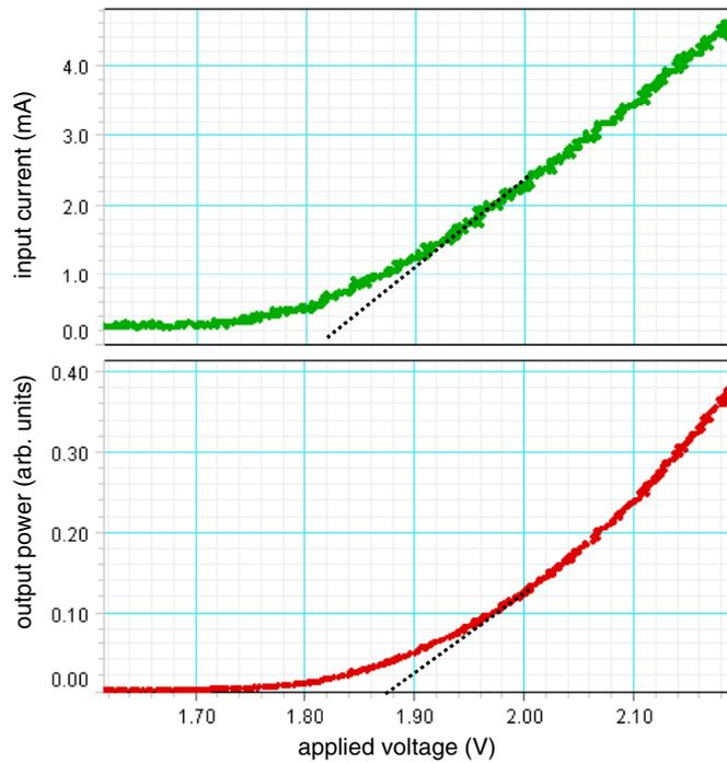
**Figure 3.** Input current and radiant output power close to the threshold of spontaneous emission. From the extrapolations, the threshold point can be taken as  $1.85 \pm 0.05$  V.
