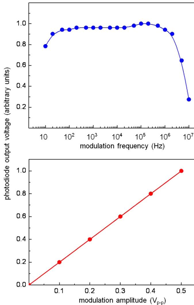
Figure 6. Modulation characteristics of the laser diode.
