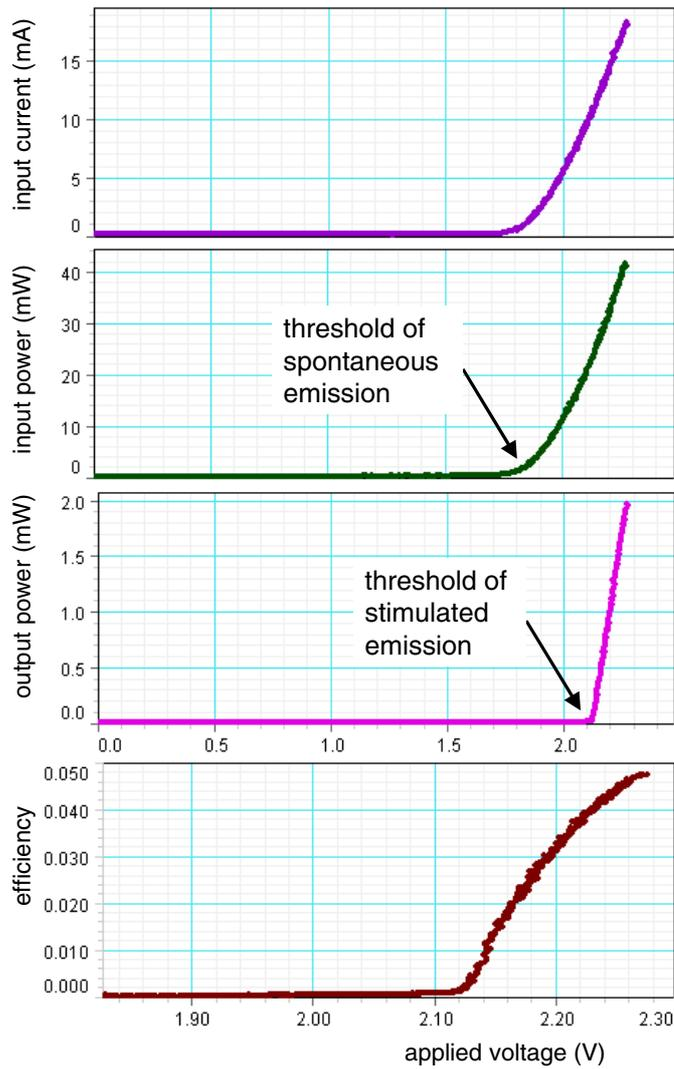
**Figure 2.** Characteristics of the laser diode versus applied voltage.
