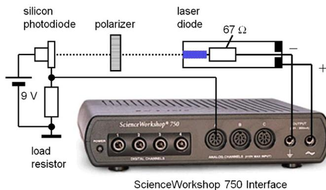
**Figure 1.** The setup with the modified laser pen, polarizer and silicon photodiode.
