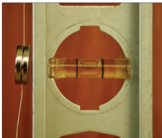
Fig. 1. Two magnets attracting each other with a thread between them do not hang vertically due to their attempt to align with the Earth's magnetic field, which is not, in general, horizontal. The level is made of aluminum (a protective cover over the bubble was removed as the screws holding it in place were magnetic).
