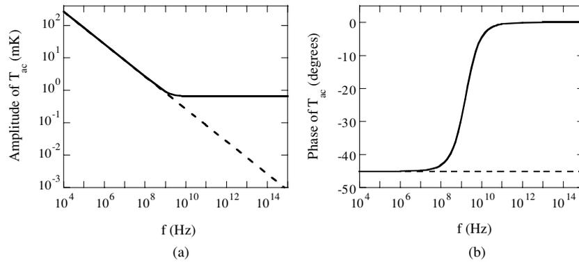
**Figure 3.** (a) Amplitude and (b) phase of the temperature oscillation on the surface of a semi-infinite stainless steel sample as a function of the modulation frequency. The solid line corresponds to the hyperbolic solution and the dotted line to the parabolic one. Calculations have been performed with  $\tau = 10^{-10}$  s and  $I_0 = 10^6$  W m $^{-2}$ .
